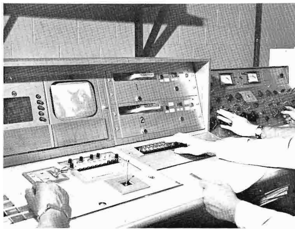
FIG. 10. Independent TS-2 delegate switcher enables technical director to select picture for previewing.
