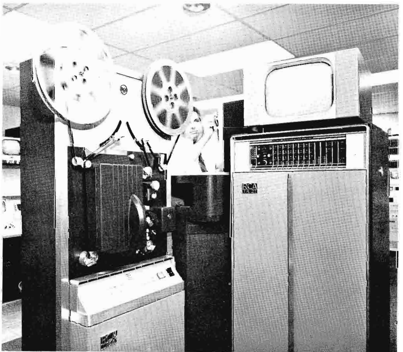
FIG. 7. Unified, New Look monitoring and control position comprising color studio and film camera controls, TS-40 switcher and special effects system, film remote controls, audio console and tape recorders.
