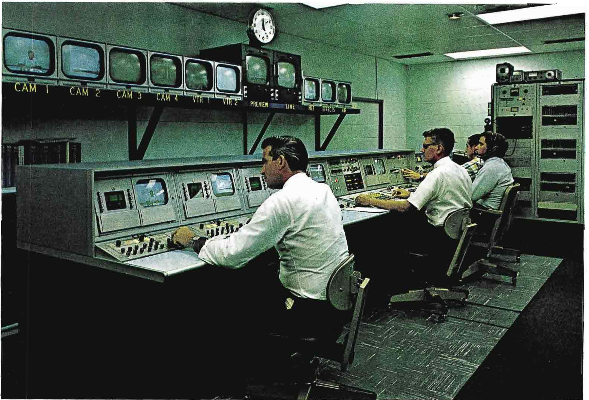
FIG. 7. Unified, New Look monitoring and control position comprising color studio and film camera controls, TS-40 switcher and special effects system, film remote controls, audio console and tape recorders.
