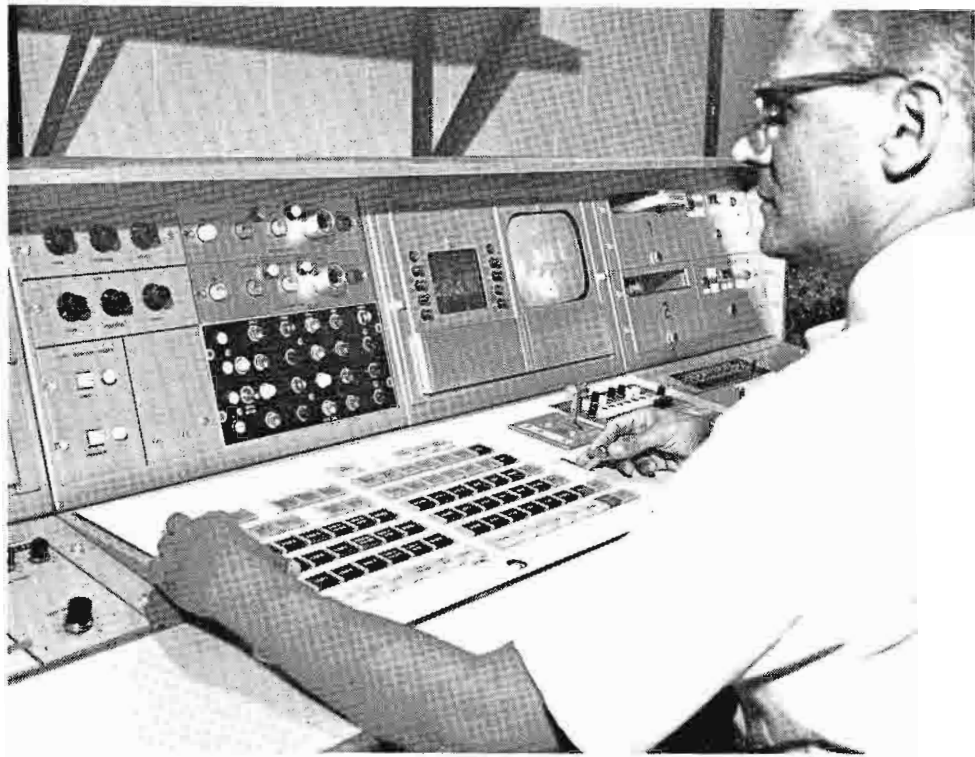
FIG. 9. Closeup view of custom TS-40 switcher and special effects panel. Above are tape and film remote controls.
